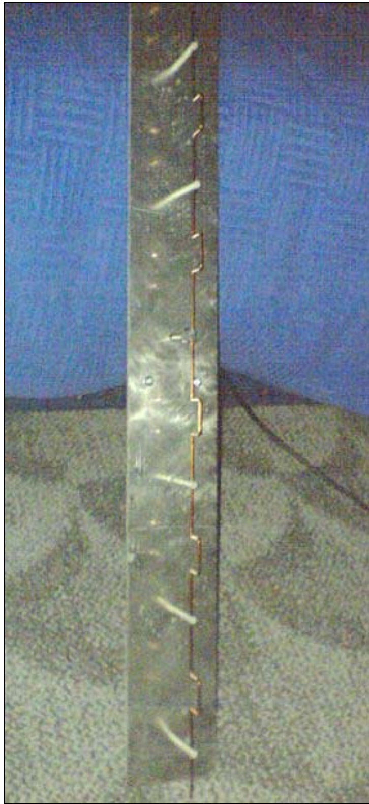
Fig. 13. Inverted Amos antenna with 7 dipoles.
