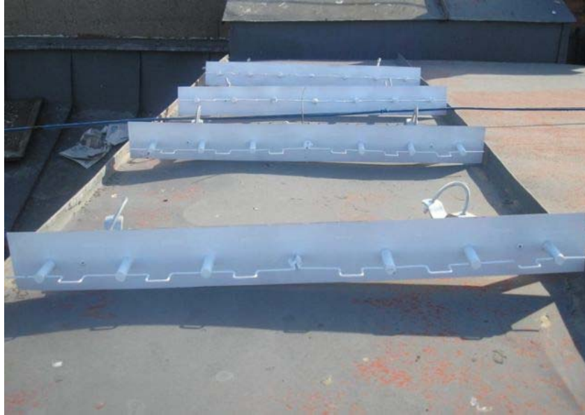
Fig. 16. Finished Inverted Amos antennas with 7 dipoles ready for mounting.
