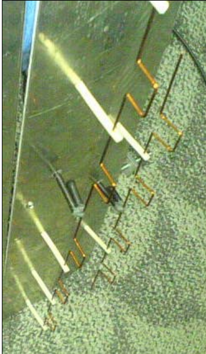
Fig. 14. Inverted Amos antennas with 5 and 7 dipoles.
