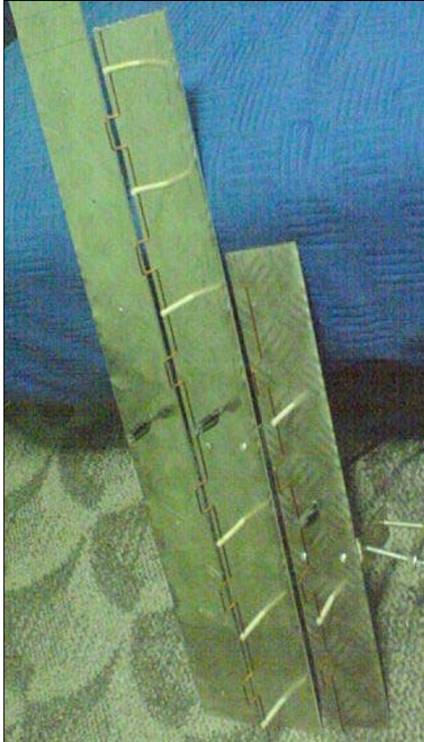
Fig. 15. Finished Inverted Amos antennas with 5 and 7 dipoles and the reflector for not yet finished antenna with 9 dipoles.
