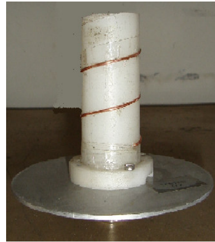
Fig (2) 2.5 Turns RHCP helical antenna at 2.4 GHz
