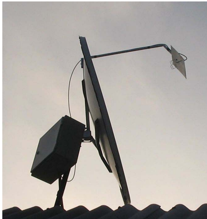
Fig. 24. Offset dish with 2 el. bi-quad feed antenna
