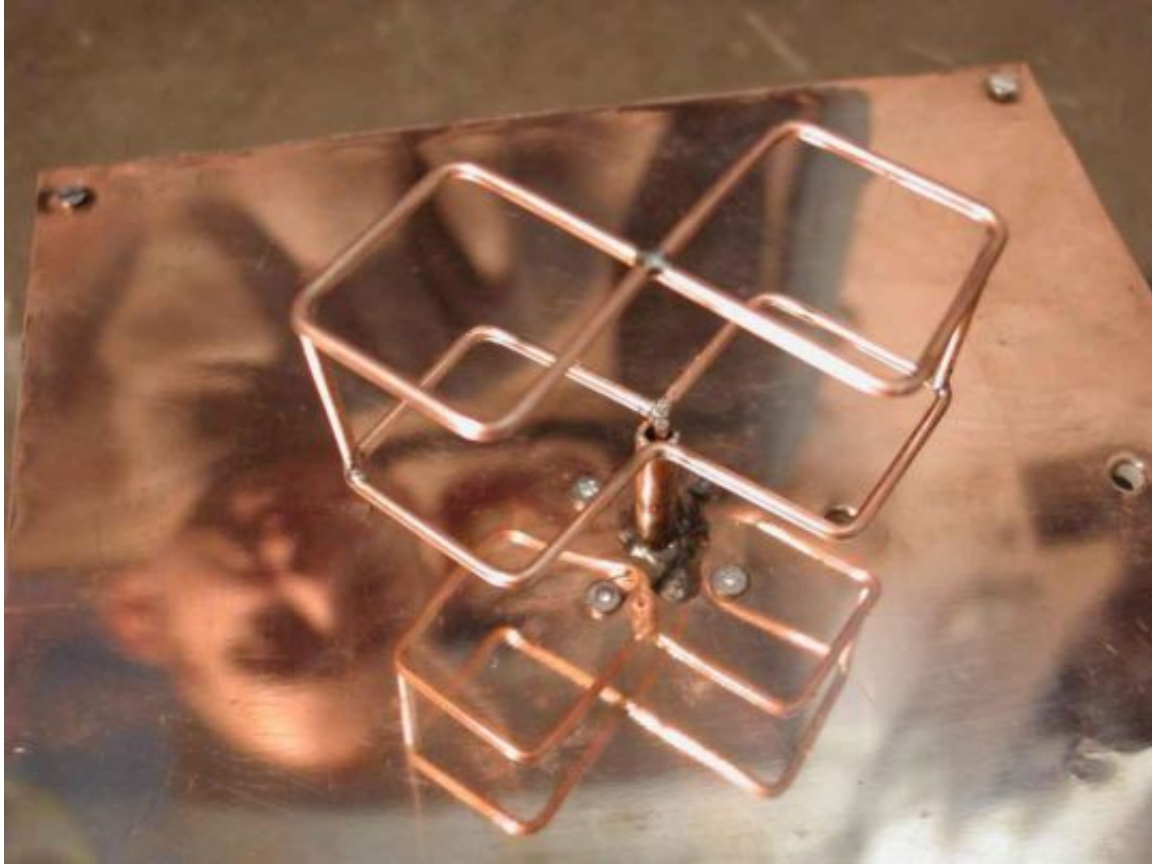
Fig. 21. Feeding of 2 el. bi-quad feed antenna
