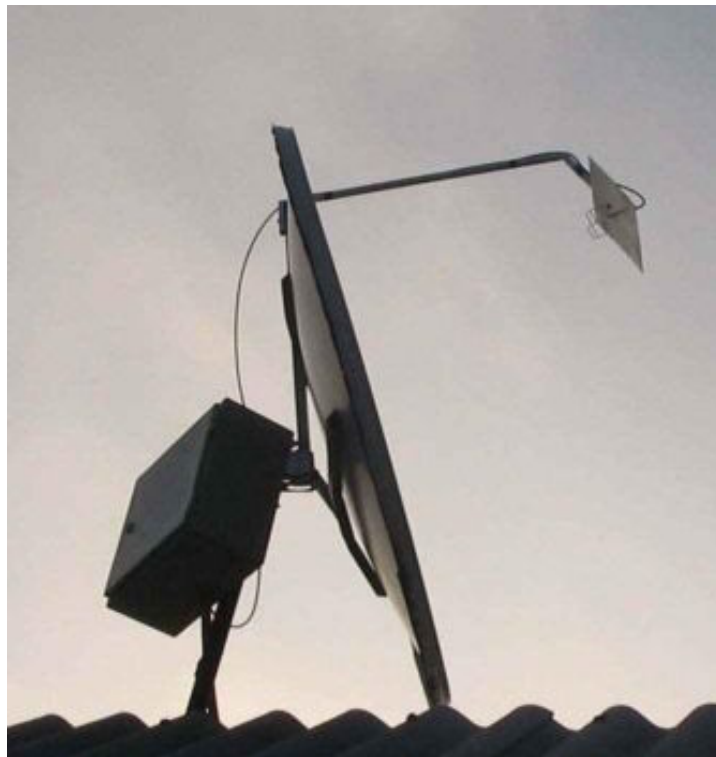
Fig. 24. Offset dish with 2 el. bi-quad feed antenna
