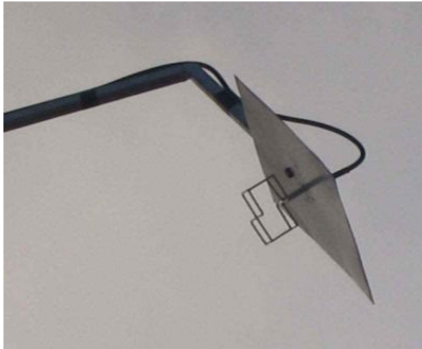
Fig. 25. Close-up view of 2 el. bi-quad feed antenna mounted on carrier
